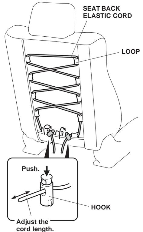
2. Install the hooks and adjust the cord length while pressing the top of the hook. Release the top to secure the cord.
