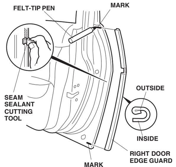
4. Position the cutting edge of the seam sealant cutting tool against the door edge, and trim the seam sealant from mark to mark, top and bottom.
