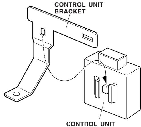
22. Inside the left rear cargo area, insert the control unit bracket through the square hole in the vehicle panel, and secure the control unit assembly with one 6 x 16 mm flange bolt.
