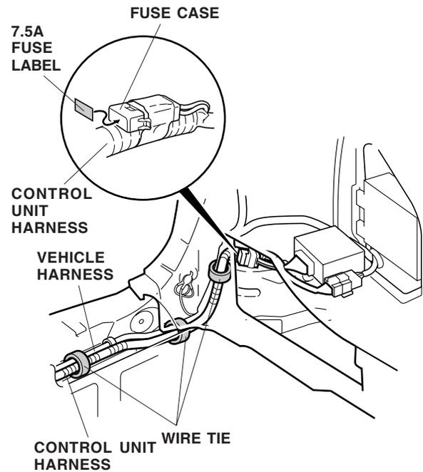
27. Route the control unit harness toward the right side of the vehicle, and secure the harness to the vehicle harness with three wire ties.
