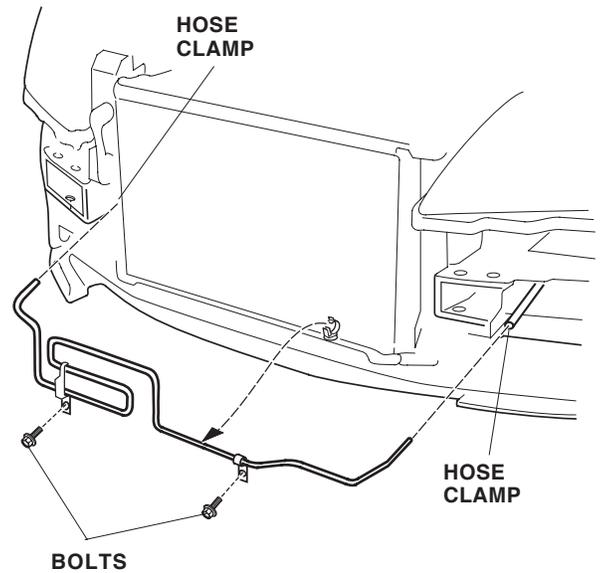
42. Install the new hose to the upper pipe of the ATF cooler, and secure the hose with one new hose clamp from the kit.
