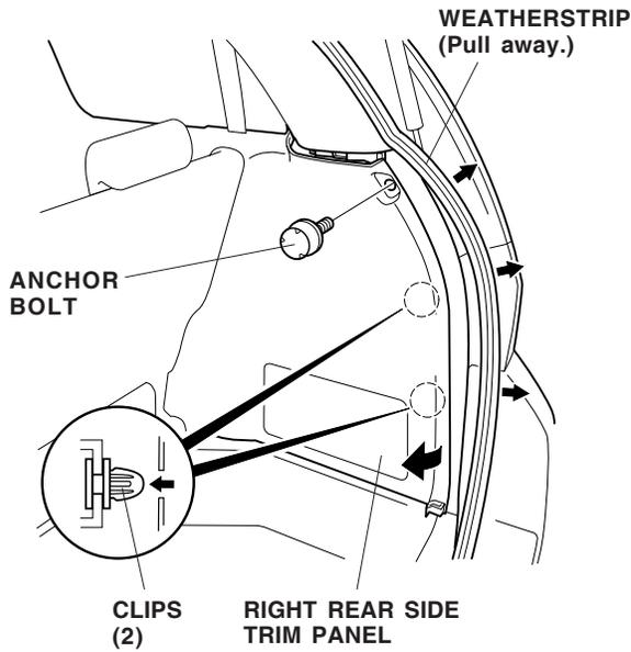
30. With an assistant gently pulling out on the right rear side trim panel, plug the control unit harness 8-pin connector into the rear junction box. Secure the control unit harness to the vehicle harness with two wire ties.
