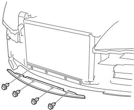
48. Reinstall the front bumper beam, and torque the bumper beam bolts to 22 lb-ft (26 N·m).
