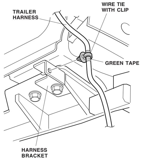
18. Secure the trailer harness to the trailer hitch with four wire ties.
