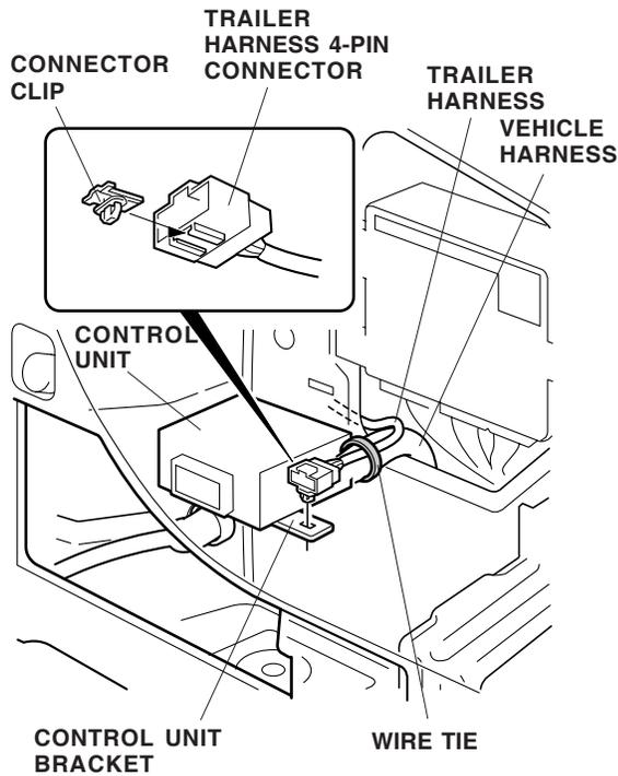
24. Secure the trailer harness with one wire tie to the vehicle harness.
