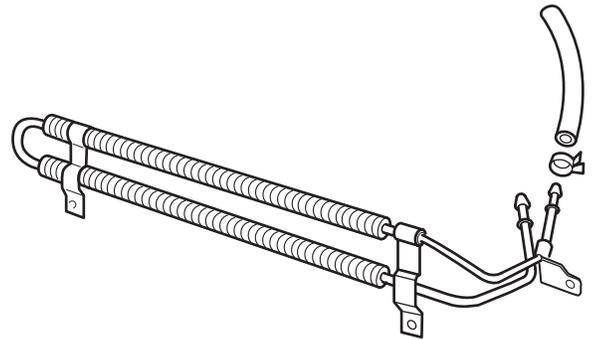
43. Locate and remove the old power steering cooler clip. Discard the clip.
