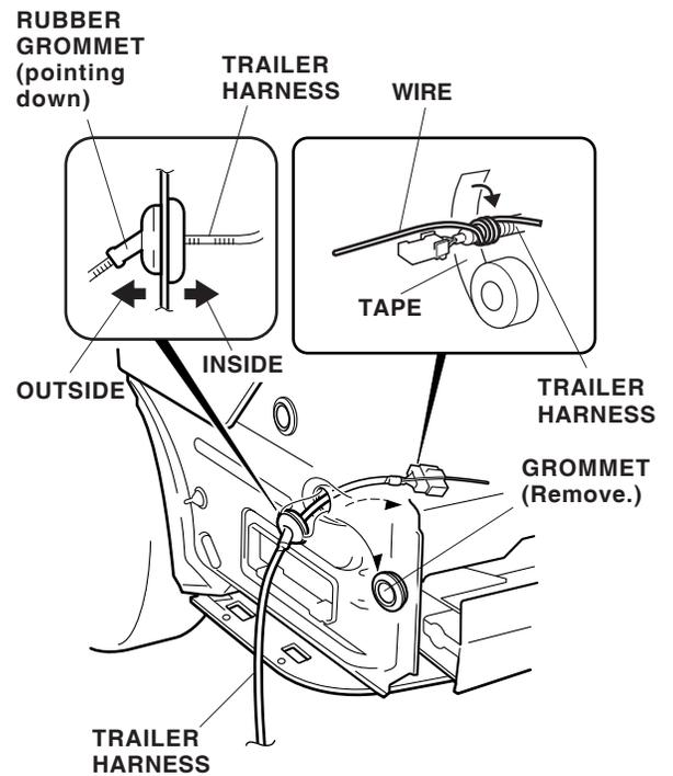
14. Tape the trailer harness to a piece of stiff wire. Route the trailer harness into the cargo area, and seat the rubber grommet into the body panel with the harness pointing down.
