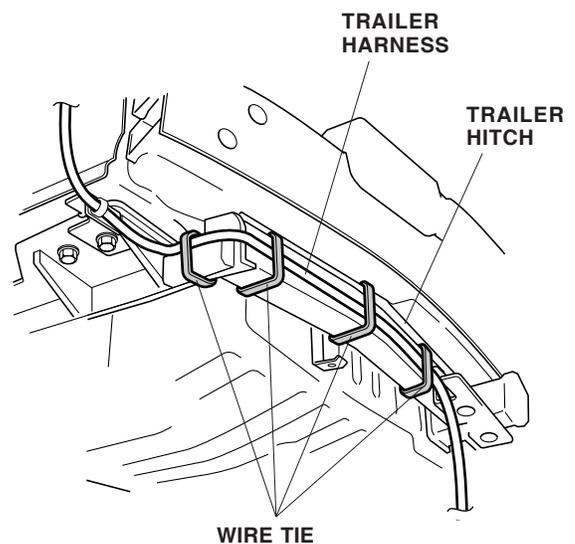
19. Insert the trailer harness 4-pin connector into the connector bracket, then attach the connector bracket to the trailer hitch with the 6 x 16 mm bolt and flange nut.
