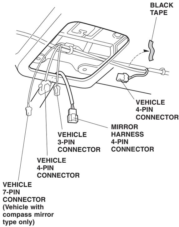
21. Plug the mirror harness 4-pin connector into the vehicle 4-pin connector.
