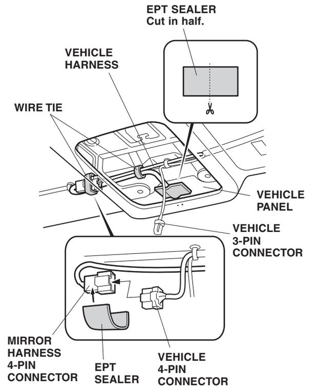
17. Cut the EPT sealer into exact halves. Wind one of the two halves of the EPT sealer you just cut onto the mirror harness 4-pin connector.
