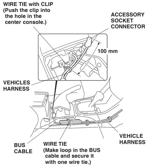
34. Check that all wire harnesses are routed properly and all connectors are plugged in.
