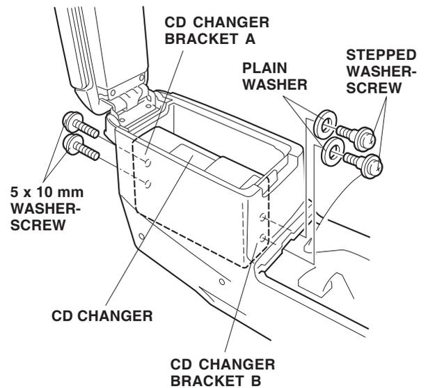
31. Secure CD changer bracket B to the center console with two stepped washer-screws and two plain washers.
