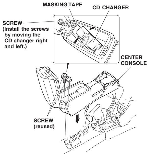
28. Reinstall the center console box inner cover with the BUS cable routed through the cutout.
