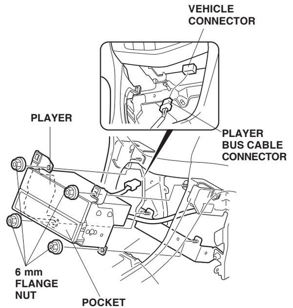
26. Route the BUS cable toward the rear along the vehicle harness, then secure the BUS cable to the vehicle harness with two wire ties.
