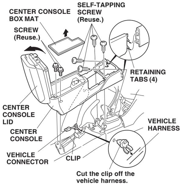
10. Remove the center console rear cover (two self-tapping screws and two clips).
