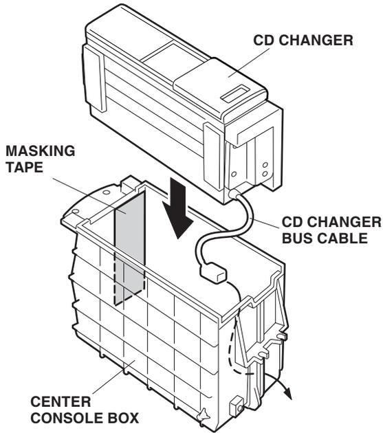
23. Reinstall the center console box into the center console using the four self-tapping screws removed in step 12.
