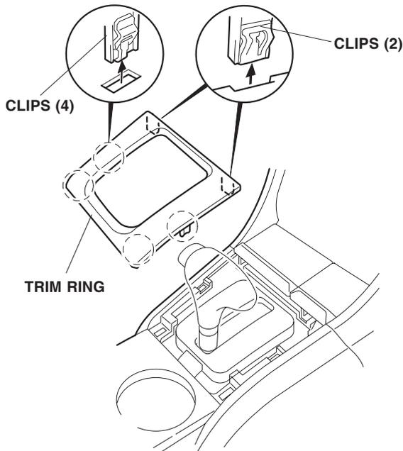
4. Pry up on the beverage holder to release the six clips, and remove the beverage holder.
