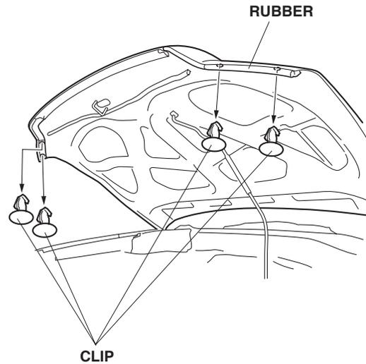
4. Turn over the rubber molding and locate the six square holes in the hood. Push one plastic grommet into each square hole.
