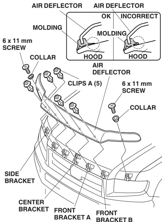
14. Aligning the holes in the air deflector over the two side brackets, install the two 6 x 11 mm screws and two collars, and then tighten the screws securely.
