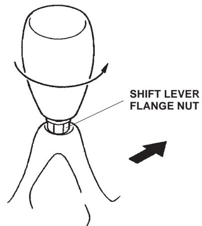
2. By hand, thread the flange nut all the way down to the last thread. Do not allow the bottom of the flange nut to extend over the last thread of the shift lever.
