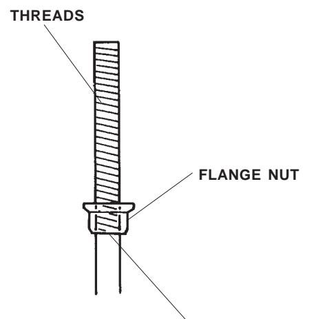
3. By hand, thread the new shift knob onto the shift lever until it bottoms against the flange nut.
