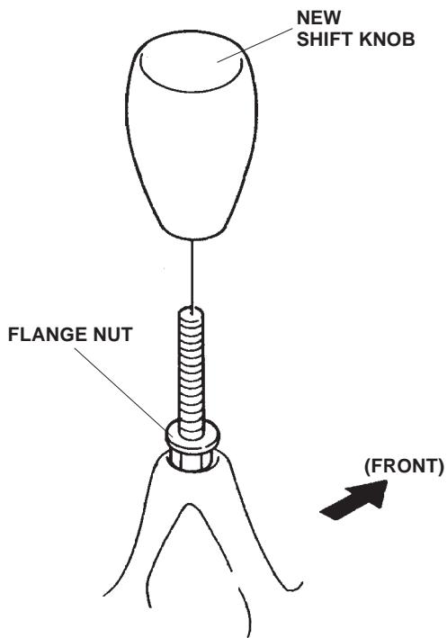
4. Turn the shift knob into the correct position for reading the gear pattern, then tighten the flange nut securely against the bottom of the shift knob using the 14 mm combination wrench.
