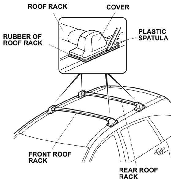
7. After installing the roof rack, rock each rack to make sure it is secure.
