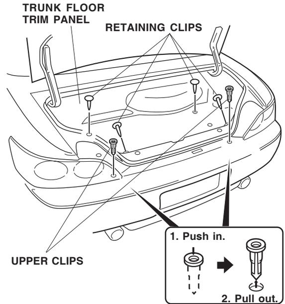
2. Remove and discard only the two upper clips that secure the rear trim panel.
