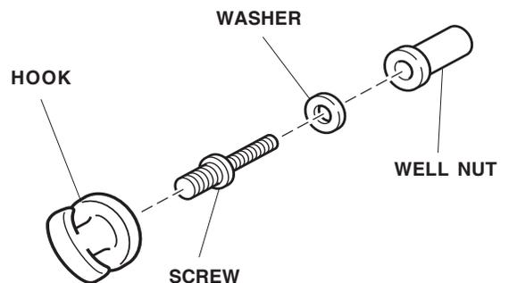
5. Install a well nut/hook assembly into each of the six holes you enlarged, and turn the hook to tighten it in place.
