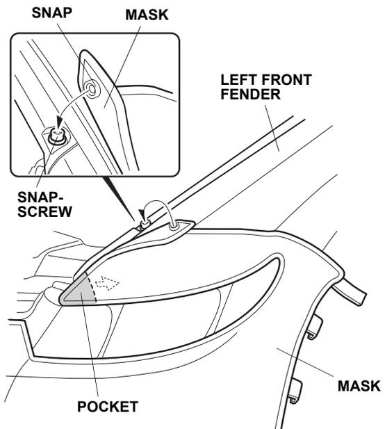
6. Attach the snap on the mask to the snap-screw you installed in step 3.
