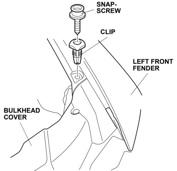
4. Repeat steps 2 and 3 to install a snap-screw on the right side of the vehicle.
