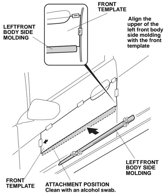
4. Align the left front body side molding with the front template and attach it to the left front door. If the vehicle has door edge film installed, align the end with the door edge film.
