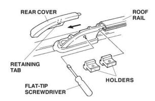
Insert two holders in the groove of the roof rail.
