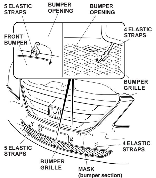
10. Hook one end of the bungee cord in the hole in the splash guard. Pass the hook of the other end of the bungee cord through the nine straps underneath the mask, and hook it in the hole in the other side of the splash guard. Insert the hooks with care so you do not shift the mask to one side.
