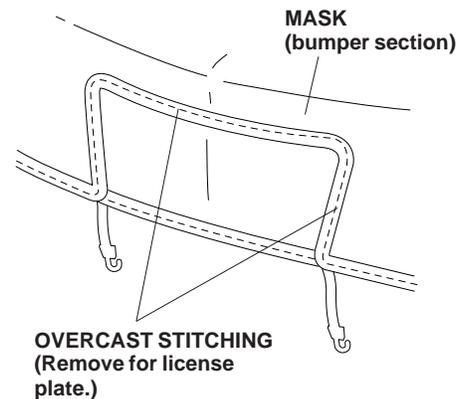
2. If the vehicle is equipped with front corner sensors, cut out the front corner sensor sections on the right and left sides of the nose mask bumper section using a utility knife.
