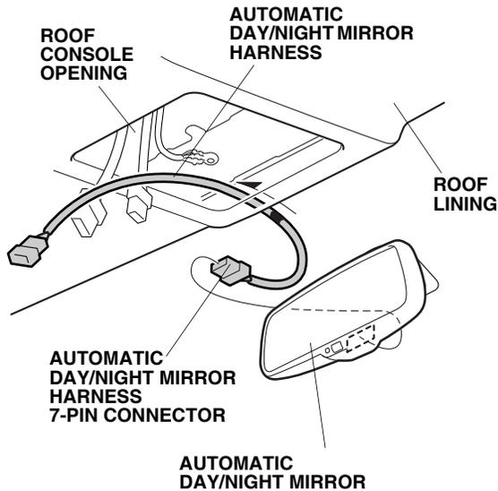
10. Align the green-taped part of the automatic day/night mirror harness with the end of the roof lining.
