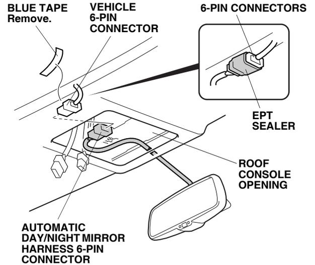
12. Wrap the EPT sealer onto the joint of the 6-pin connectors.
