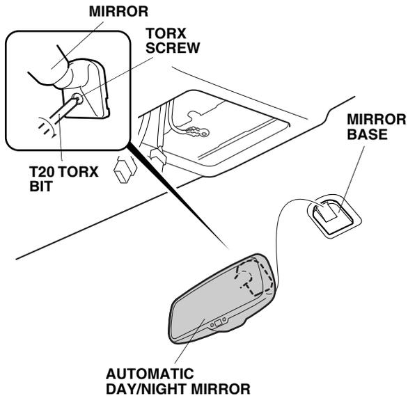
9. Plug the automatic day/night mirror harness 7-pin connector to the automatic day/night mirror. Route the automatic day/night mirror harness as shown.
