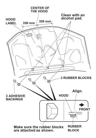
6. Remove the adhesive backings from three rubber blocks and hood label and attach them to the hood as shown.
