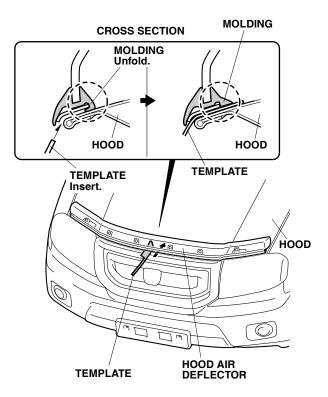
15. Open the hood. Tighten the four truss screws loosely tightened in step 4.
