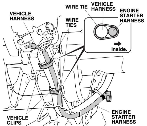
33. Disconnect the vehicle 20-pin connector from the TPMS control unit (removed in step 24) and plug it into the engine starter harness 20-pin connector. Plug the remaining engine starter harness 20-pin connector into the TPMS control unit.
