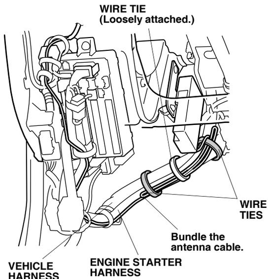
73. Secure the antenna cable to the engine starter harness with two additional wire ties.
