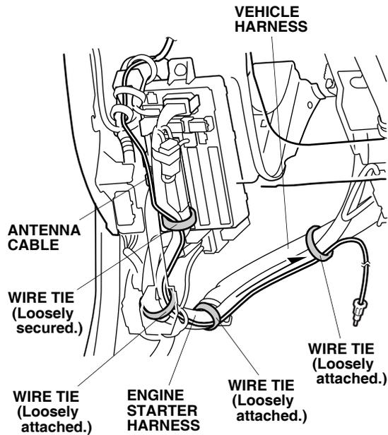
64. Secure the antenna cable to the engine starter harness with the four wire ties you loosely attached.
