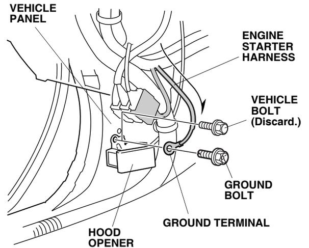
46. Secure the engine starter harness to the vehicle harness with one wire tie.
