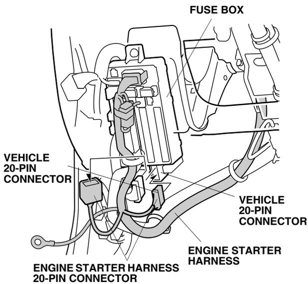
44. Attach the clip from the engine starter harness connector to the clip on the vehicle connector.
