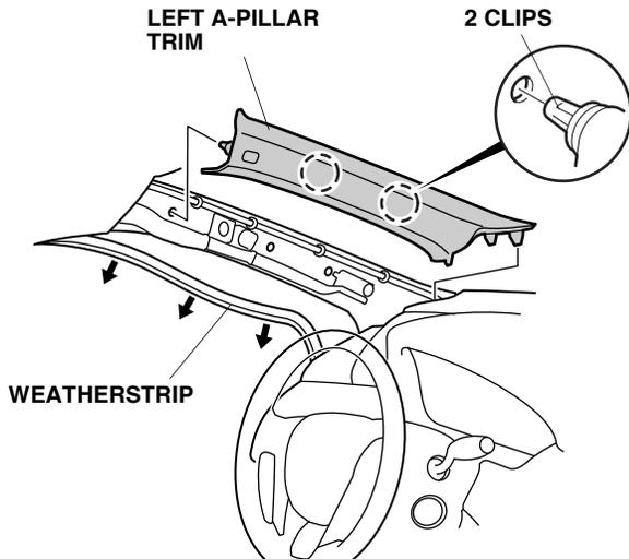
19. Remove and discard the clip from the left front A-pillar trim, and install a new A-pillar clip (supplied) on the left front A-pillar trim.
