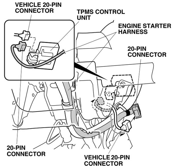
34. Align the green tape on the engine starter harness with the clip on the vehicle harness, and secure the engine starter harness to the vehicle harness with one wire tie.
