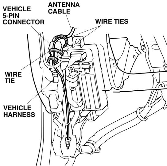
62. Secure the antenna cable with two wire ties to the vehicle harness.
