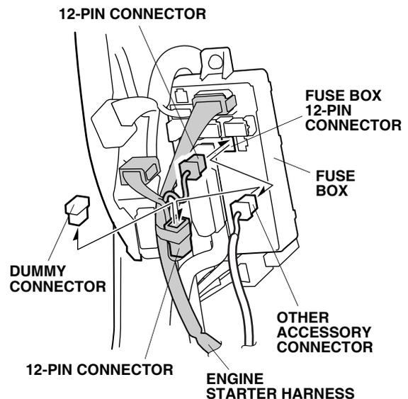
42. Loosely attach the engine starter harness to the vehicle harness with one wire tie.
