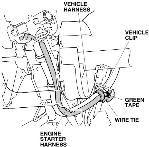
35. Near the connector, secure the engine starter harness to the vehicle harness with one wire tie.
