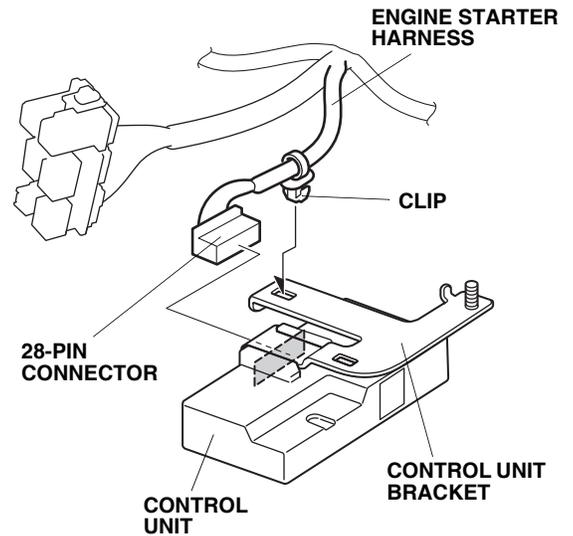
67. Install the clip from the engine starter harness to the control unit bracket.
