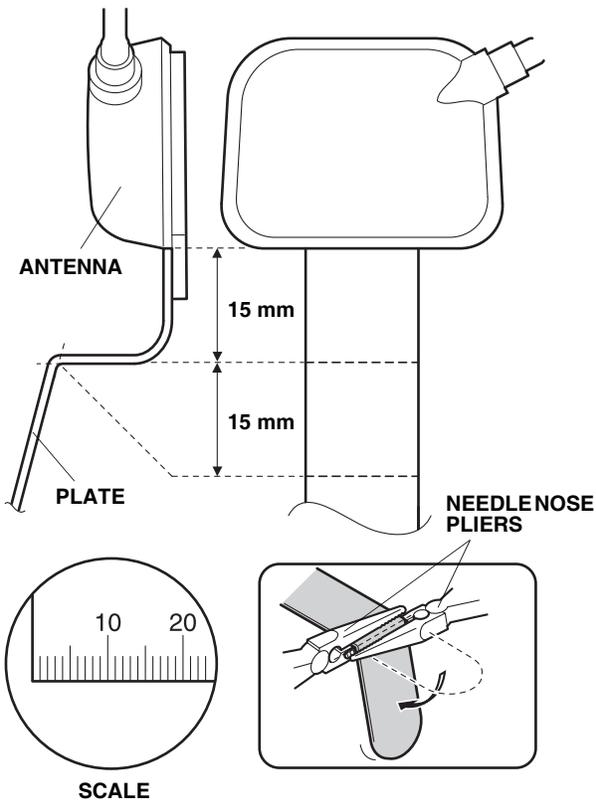
51. Starting near the antenna end of the cable, wrap urethane tape around the antenna cable at the measurements shown.
