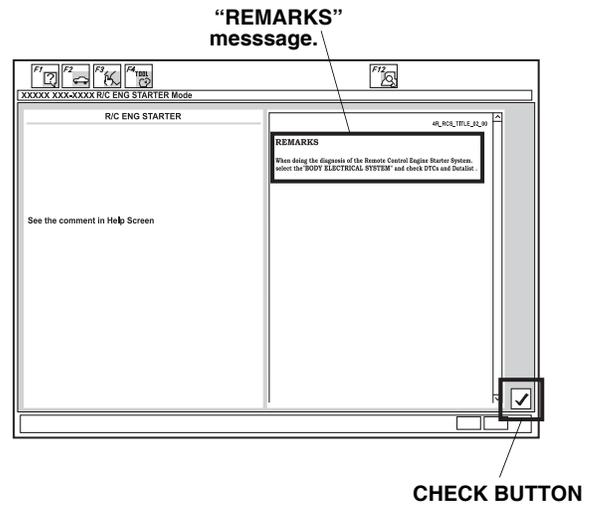
8. Select **REGISTER REMOTE CONTROL ENGINE STARTER UNIT**, then click the check button.
