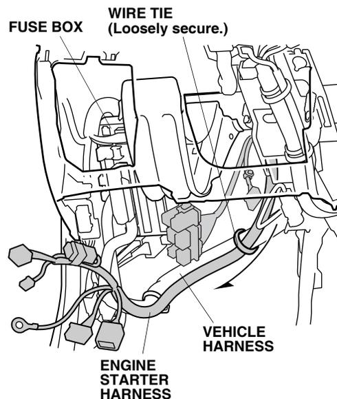
40. Disconnect the vehicle 5-pin connector from the fuse box. Plug the engine starter harness 5-pin connector into the fuse box 5-pin connector. Wrap one urethane tape around the vehicle 5-pin connector. NOTE: Check that the engine starter harness 5-pin connector is connected to the vehicle connector and locked securely. A loose connector can cause the engine to stall.
