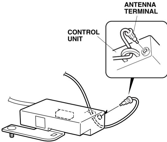
69. Secure the control unit to the vehicle frame using the flange nut.
