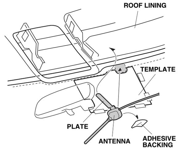
55. Remove the adhesive backing from the antenna. Insert the antenna plate over the roof liner, and attach the antenna to the front window aligning it with the template.
