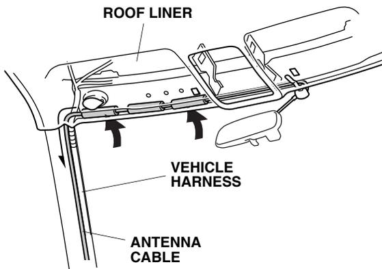
58. Using scissors, cut one urethane tape in half. Route the antenna cable towards the driver's side of the vehicle, and secure the antenna cable to the roof panel with the two halves of urethane tape.
