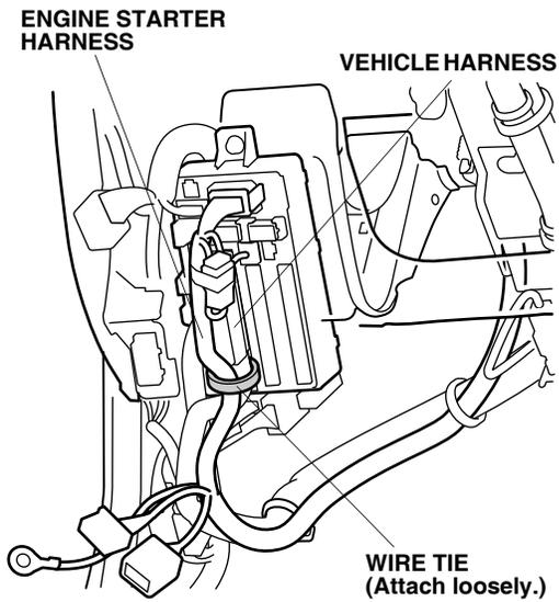
43. Disconnect the vehicle 20-pin connector from the fuse box, and plug it into the engine starter harness 20-pin connector. Plug the remaining engine starter harness into fuse box 20-pin connector.
