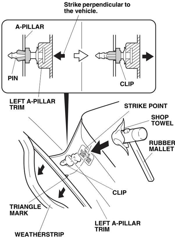
17. Using a small rubber mallet and a shop towel, gently tap the left A-pillar trim at the position shown to release the clip.
