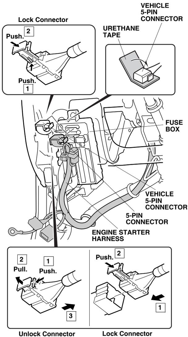
41. Plug the engine starter harness 12-pin connector into the fuse box 12-pin connector.
