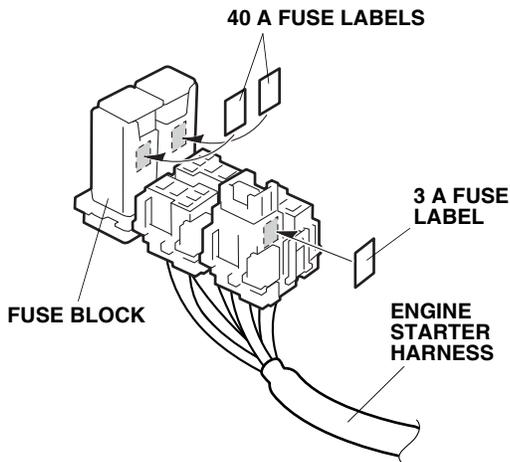
22. Attach the 3 A fuse label to the engine starter relay block.
