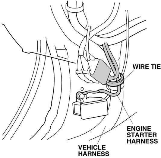
47. Loosely attach the engine starter harness to the vehicle harness with two wire ties.
