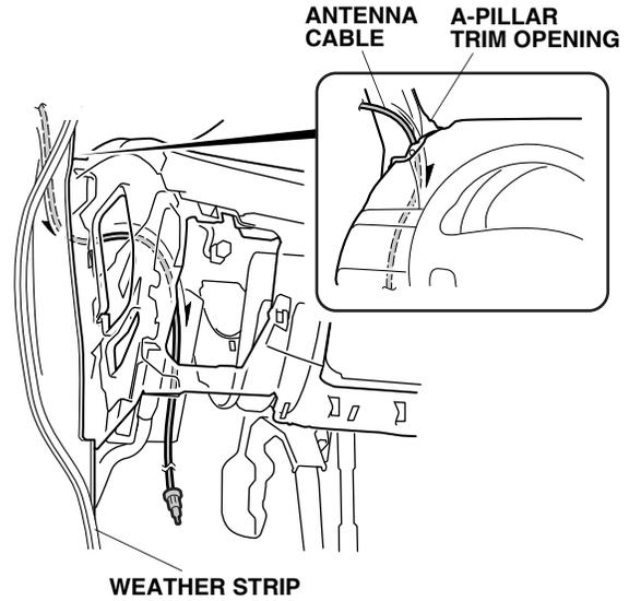
60. Secure the antenna cable to the vehicle harness with four wire ties.
