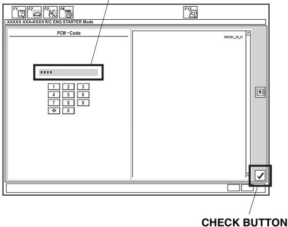
11. The following message will display: **The registration of the Remote Control Engine Starter Unit has been completed.** Click on the check button.
