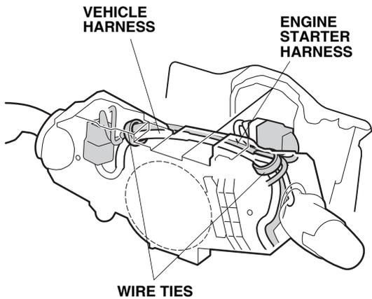
32. Secure the engine starter harness to the vehicle harness with two wire ties in the areas shown.
