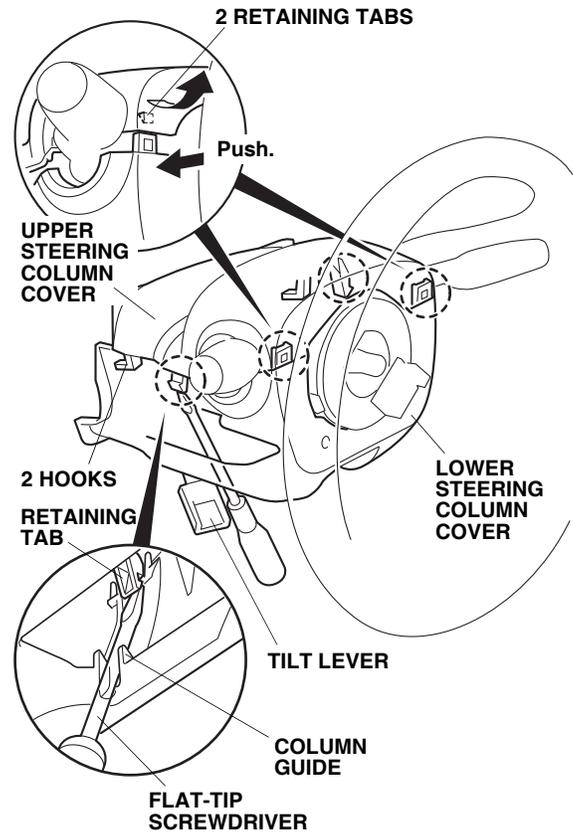
12. Remove the lower steering column cover (three screws). The upper screws are self-tapping screws.
