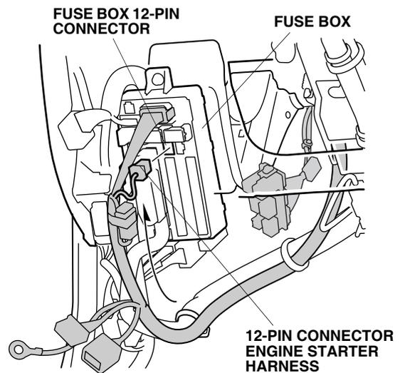
NOTE: If the 12-pin connector is already being used, unplug the 12-pin connector from the fuse box, and plug the engine starter harness 12-pin into the fuse box. Remove and discard the dummy connector from the engine starter harness and plug 12-pin connector into the engine starter harness.
