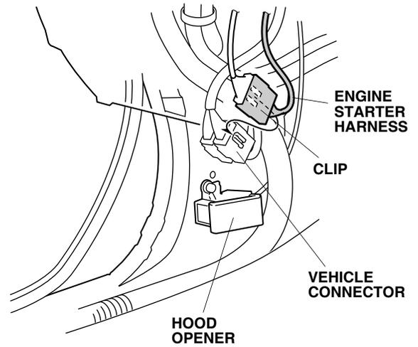
45. Remove and discard the upper hood opener bolt, and install the ground bolt supplied with the ground terminal attached.
