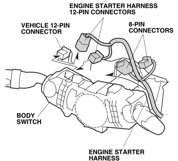
30. Disconnect the vehicle 8-pin connector and plug it into the engine starter harness 8-pin connector. Plug the remaining engine starter harness 8-pin connector into the wiper switch.
