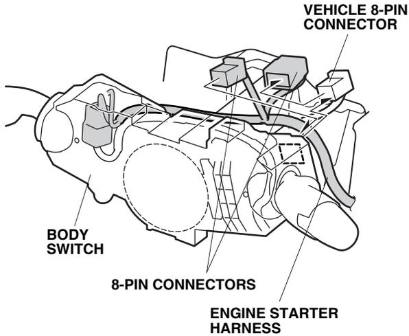
31. Secure the engine starter harness to the vehicle harness using two wire ties. Do not secure to the SRS harness.
