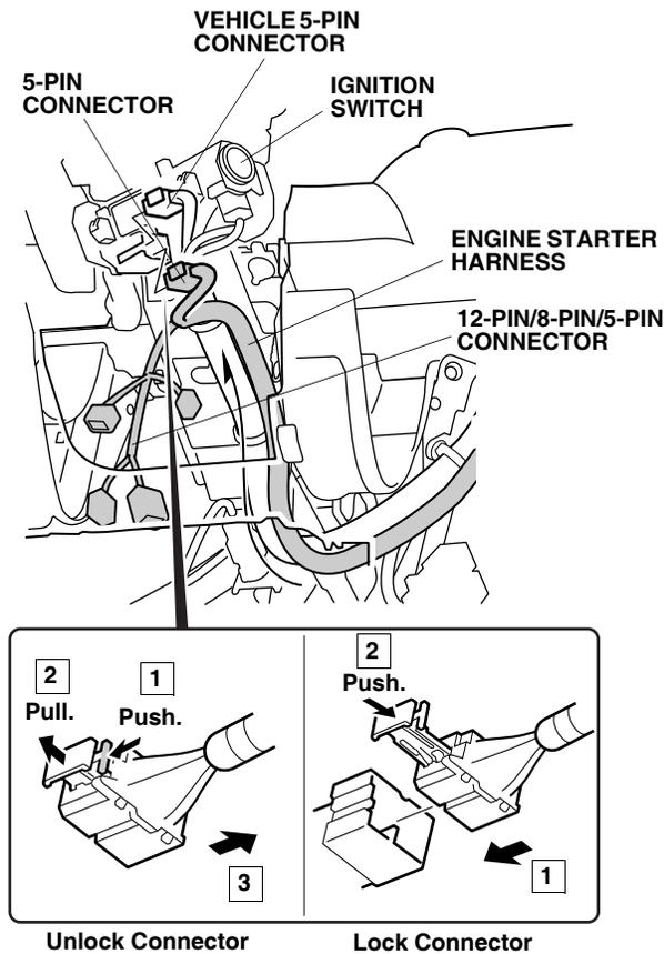
27. Disconnect the vehicle 5-pin connector from the ignition switch, and plug the engine starter harness 5-pin connector into the ignition switch.
