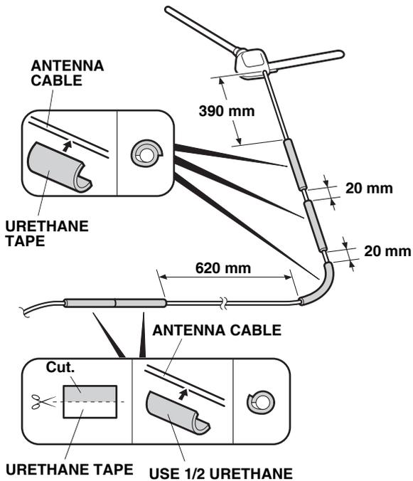
52. Using scissors, cut one urethane tape in half. Wrap the two halves of the urethane tape around the antenna cable at the measurements shown.
