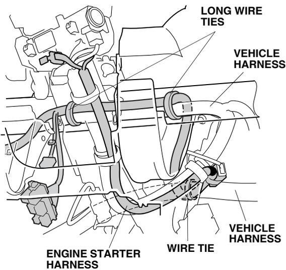
36. Secure the engine starter harness to the vehicle harness with two long wire ties at the locations shown.
