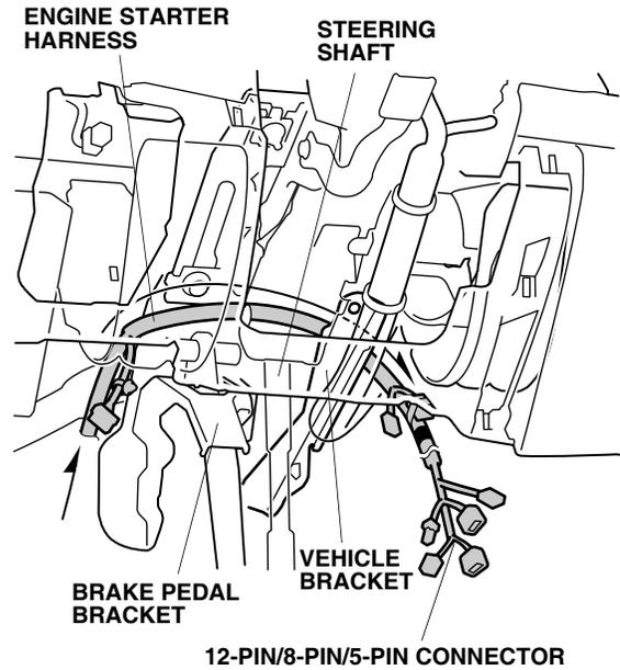
26. Route the 12-pin/8-pin/5-pin connector end of the engine starter harness to the ignition switch.
