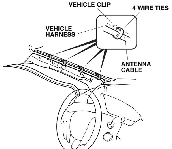
61. Secure the vehicle 5-pin connector (disconnected in step 40) to the vehicle harness with one wire tie.
