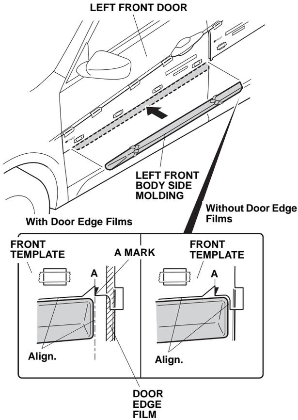
10. Press the left front body side molding firmly with the palm of your hand and remove the adhesive backing 50 to 100 mm (2 to 4 in.) at a time.
