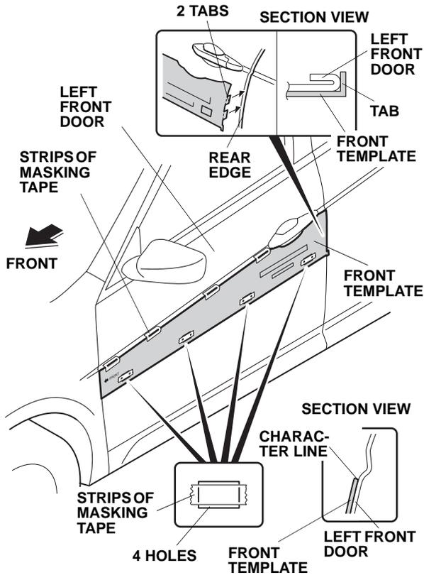
3. Align the front template with the character line on the left front door, and attach the front template to the left front door using strips of masking tape.
