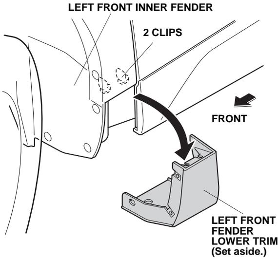
4. Remove the two clips that fasten the lower left front fender panel.
