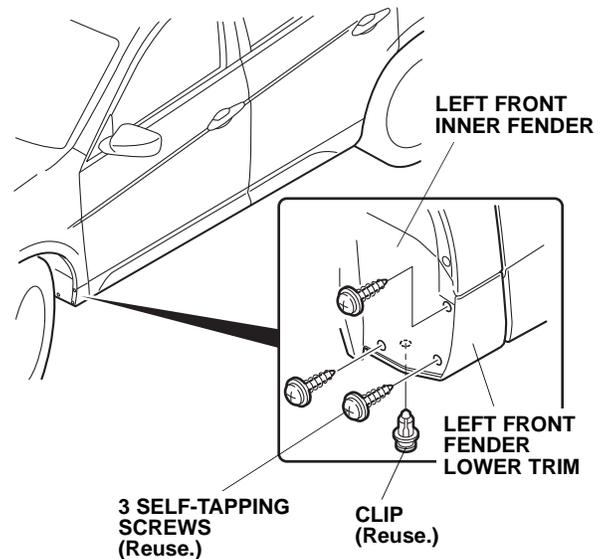
2. Remove the three self-tapping screws and one clip from the left front fender lower trim.
