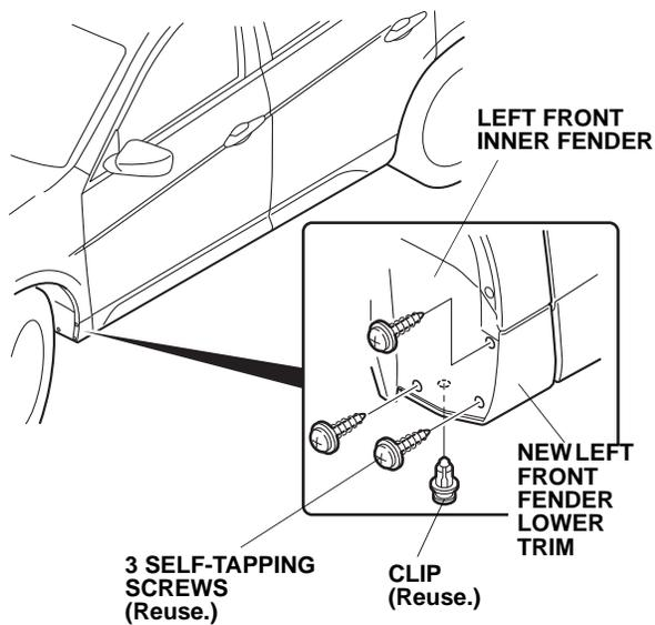
17. Secure the new left front fender lower trim using three self-tapping screws and one clip.
