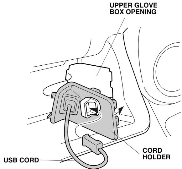
20. With the center panel near the dashboard, plug the USB cord connector into the control unit. Plug in all the vehicle connectors and reinstall the center panel.
