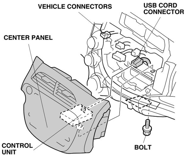
21. Check that all wire harnesses and cables are routed properly and that all connectors are plugged in.
