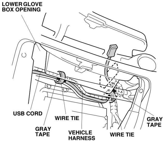
17. Using two wire ties, secure the USB cord to the vehicle harness in the areas shown.
