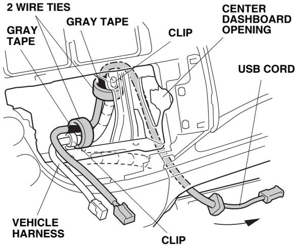
15. Using two wire ties, secure the USB cord to the vehicle harness in the areas shown.
