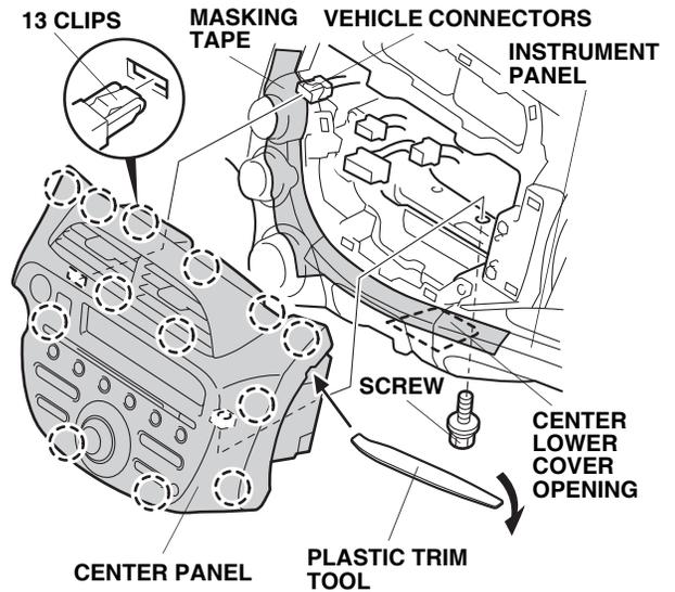
9. Remove the one screw. Using a plastic trim tool, pull the center panel out toward you to release the 13 clips. Unplug the vehicle connectors to remove the center panel.
