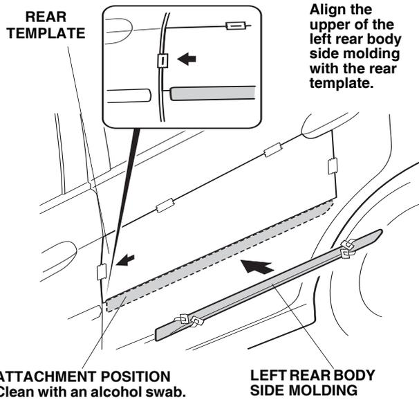
11. Align the left rear body side molding with the rear template and attach it to the left rear door.
