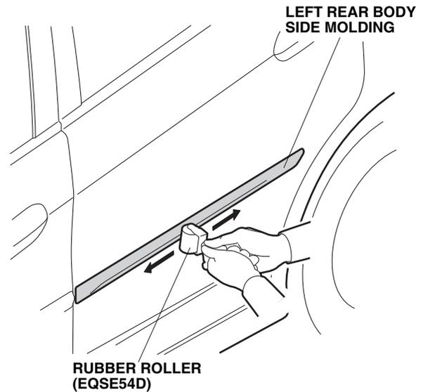
15. Turn the templates over and repeat steps 1 thru 14 to install the body side moldings on the right side of the vehicle.
