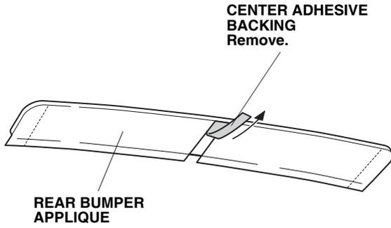
3. Place the rear bumper applique on the rear bumper, and align the cutout tailgate latch anchor. Be sure the rear bumper applique is aligned with the end of the curved surface.
