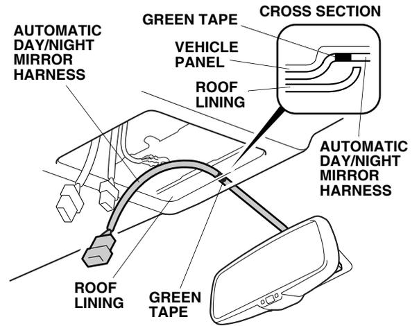
11. Locate the vehicle 6-pin connector and remove a blue tape from the vehicle 6-pin connector. Plug the automatic day/night mirror harness 6-pin connector to the vehicle 6-pin connector.
