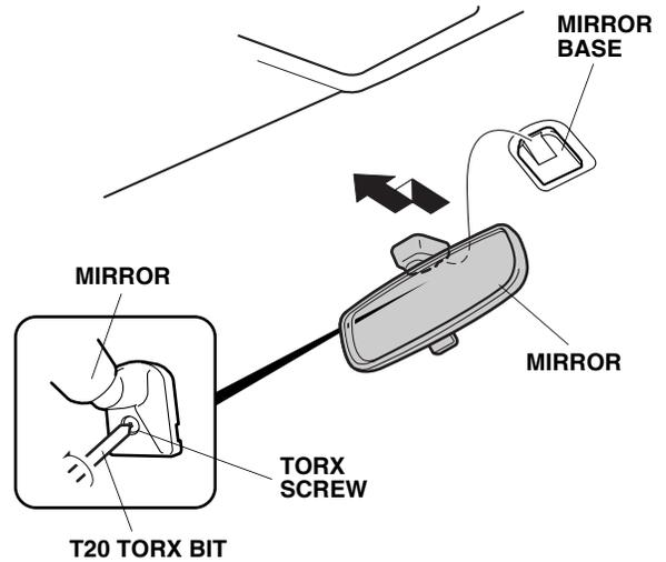
8. Install the automatic day/night mirror on the mirror base as shown, and tighten the Torx screw.
