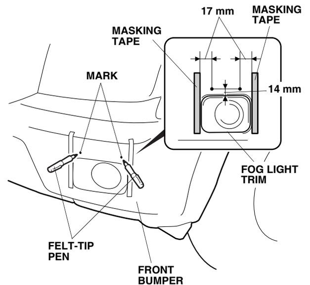
2. Using a scale and a felt-tip pen, measure and mark two locations on the front bumper.
