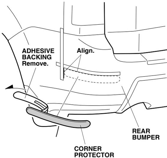
18. Attach the corner protector to the rear bumper by aligning it with the masking tapes.
