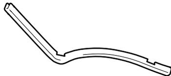
Seam sealant cutting tool
