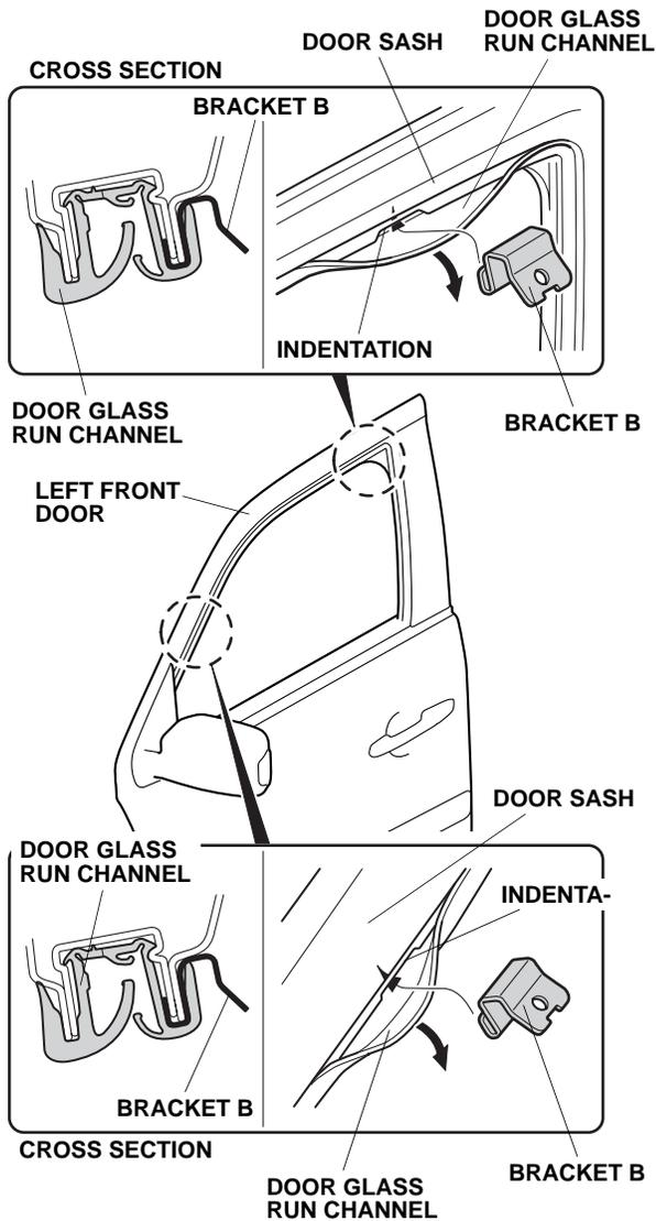
2. Peel the door glass run channel and install two brackets B to the left front door as shown. Make sure that the brackets are installed in the correct position. Check that the brackets and the door glass run channel is installed on the door sash properly.
