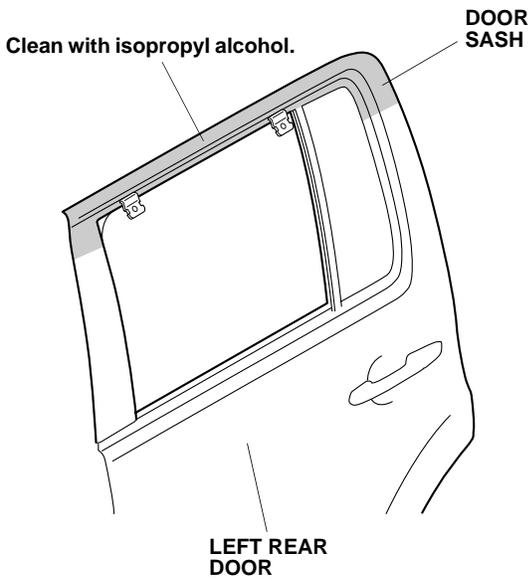
14. Align the holes on two brackets C to the holes on the left rear door visor and secure it with two rivets.
