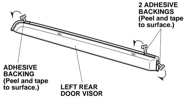
13. Using the isopropyl alcohol on a shop towel, clean the door sash where the left rear door visor will attach.
