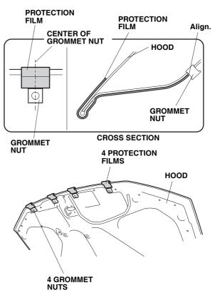
3. Remove the adhesive backings from the protection films and attach four protection films around the front of the hood as shown.
