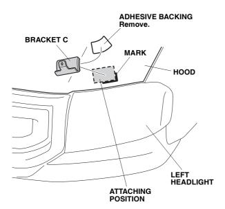
11. Reverse the template and repeat steps 7 through 10 for the bracket C on the right side of the vehicle.
