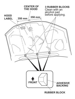
6. Remove the adhesive backings from three rubber blocks and hood label and attach them to the hood as shown.
