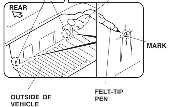
2. Under the rear of the vehicle, locate and mark the center of each concave on the outside of the trunk with a felt-tip pen.
