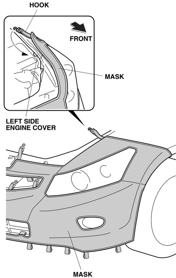
13. Attach two hooks to the edge of the radiator cover.
