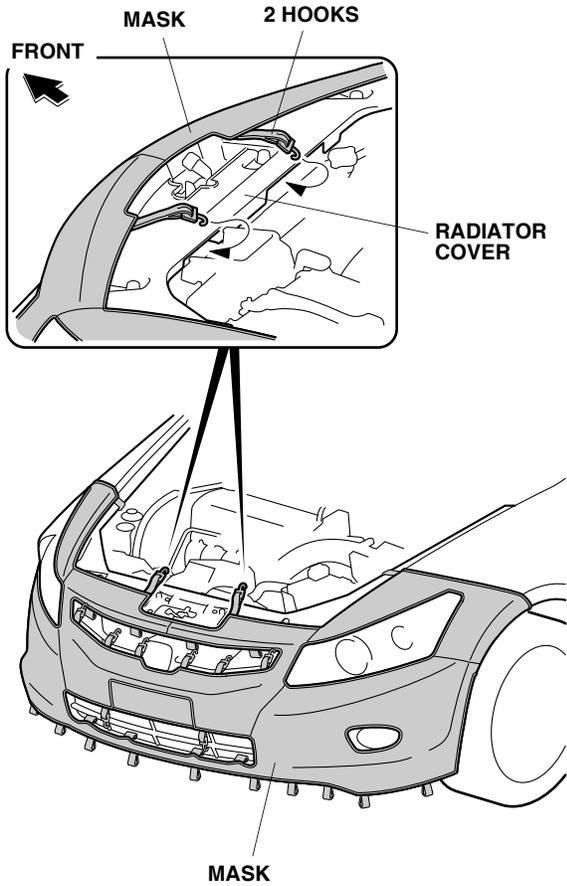
14. Attach four plastic hooks to the inside edge of the front bumper.
