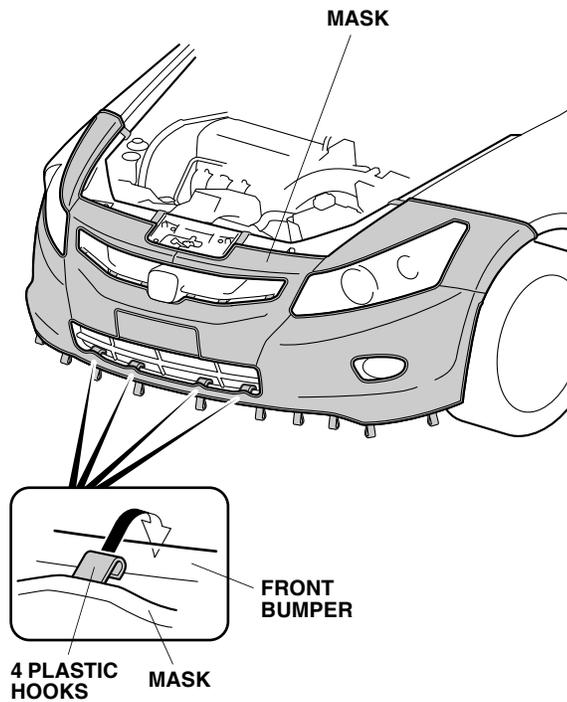
18. Route the elastic cord through the twelve loops on the bottom of the mask. Attach one hook to the hole in the inner fender. Stretch the elastic cord and attach the other hook to the inner fender hole on the other side.
