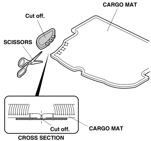
2. Open the hatch, and place the cargo mat on the cargo floor as shown.
