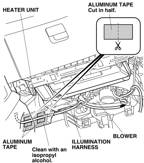
51. Using scissors, cut one aluminum tape in half. Secure the illumination harness to the back of the heater unit with two pieces of aluminum tape as shown.
