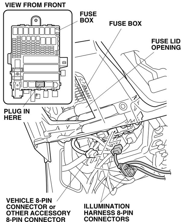
38. Plug the vehicle 8-pin connector or other accessory 8-pin connector into the illumination harness 8-pin connector.
