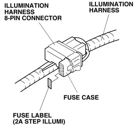
37. Unplug the vehicle 8-pin connector or other accessory 8-pin connector (if equipped) from the fuse box, and plug the illumination harness 8-pin connector into the fuse box.
