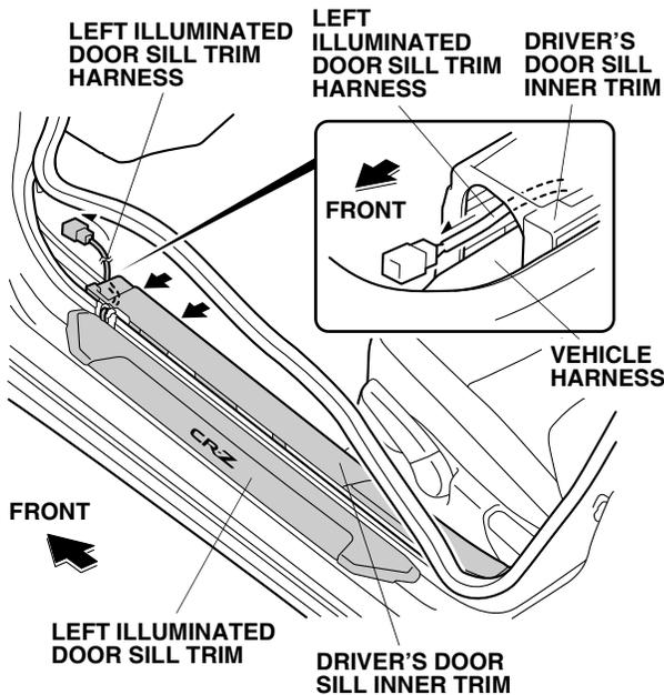
33. Reinstall the driver's door sill inner trim and door seal.
