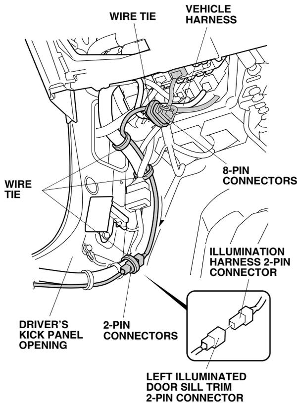
40. Secure the 8-pin connectors to the vehicle harness with one wire tie.
