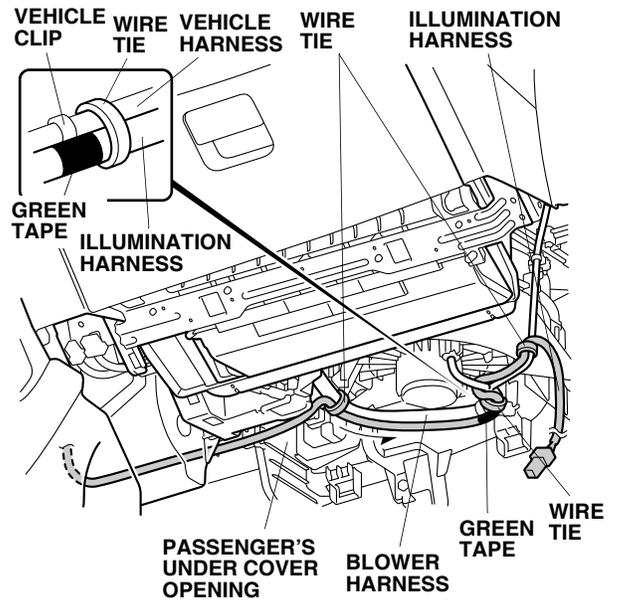
48. At the green tape, secure the illumination harness to the vehicle clip, and secure the illumination harness to the blower harness with one wire tie.
