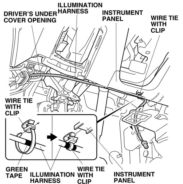
43. Attach one wire tie with clip to the green tape on the illumination harness, and secure it to the instrument panel.
