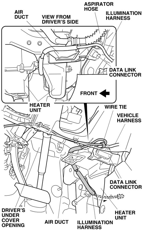
46. Secure the illumination harness to the vehicle harness with one wire tie.
