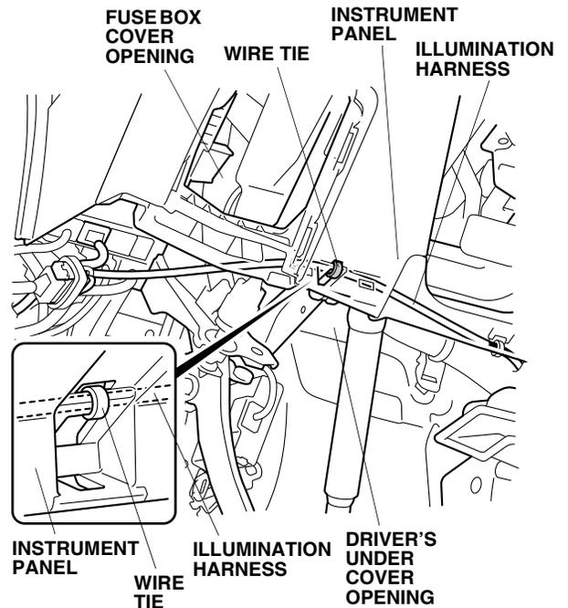
45. Route the illumination harness to the passenger side of the vehicle as shown.
