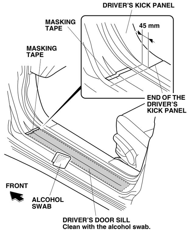
2. Using one alcohol swab, thoroughly clean the door sill where the driver's door sill trim will attach.
