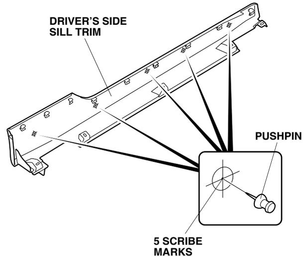
5. While wearing eye protection, drill the five holes made on the driver's side sill trim with a 3 mm drill bit, then finish with a 6 mm drill bit. Remove any burrs.
