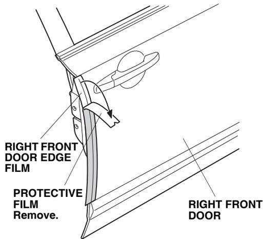
11. Starting from the middle and working outward, fold back the right front door edge film onto the inside edge of the right front door as shown. Move your fingers in one direction only.
