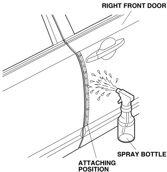
4. Using a spray bottle with 3M protective tape application solution, spray the area where the right front door edge film will attach.
