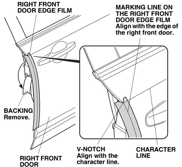
7. While slowly removing the backing on the backside of the right front door edge film, attach the right front door edge film to the right front door securely. Align the marking line on the right front door edge film with the edge of the right front door.
