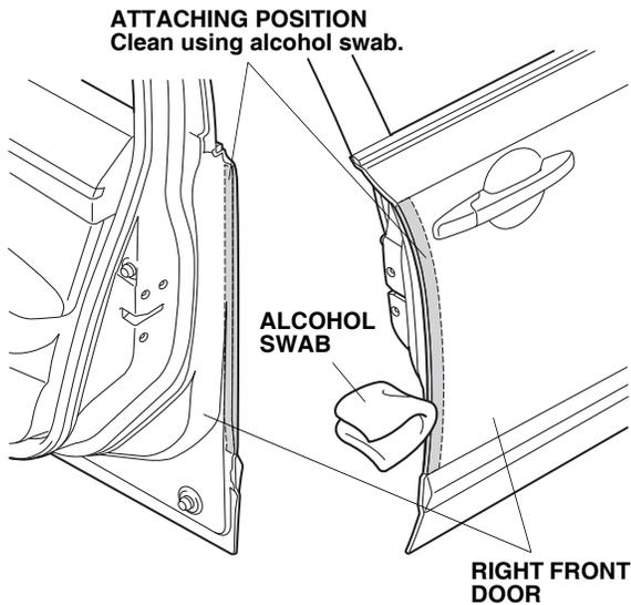
2. Using an alcohol swab, thoroughly clean the area where the right front door edge film will attach.
