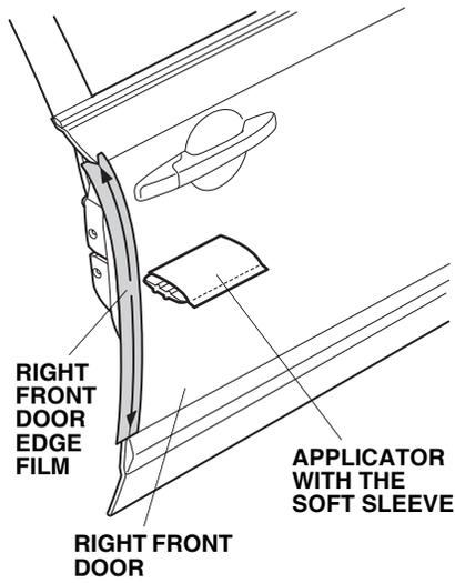
9. Starting from the middle and working outward, use the applicator to smooth the right front door edge film. Move the applicator in one direction only.
