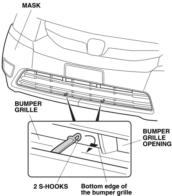
13. Route the elastic cord through the ten loops on the bottom of the mask. Attach one S-hook to the bottom edge of the bumper on one side. Stretch the cord, then attach the other S-hook to the bottom edge of the bumper on the other side.
