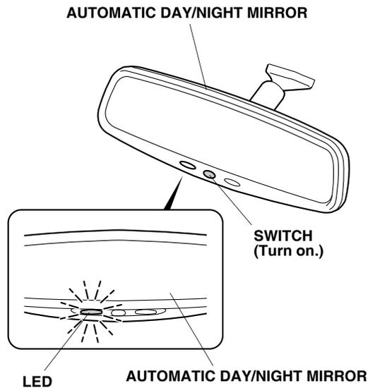
2. Turn the automatic day/night mirror switch on. Check that the LED comes on.
