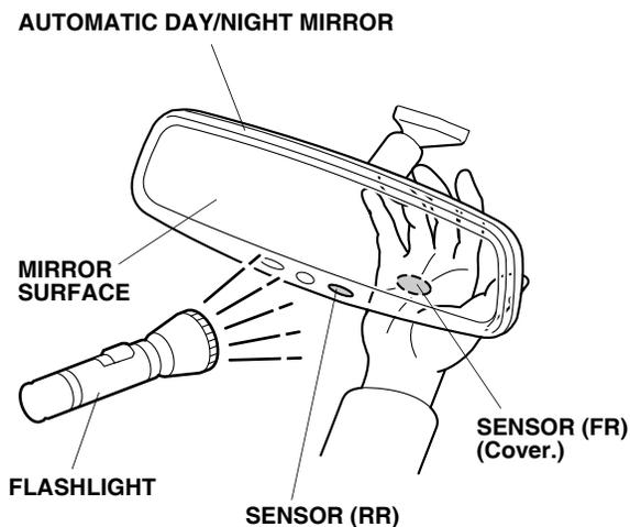
4. With the parking brake applied, press on the brake pedal, and move the select lever to the "R" position. Repeat step 3, and check that the mirror surface does not dim when in the "R" position. If the automatic day/night mirror does not function properly, check the fuse and all connectors.
