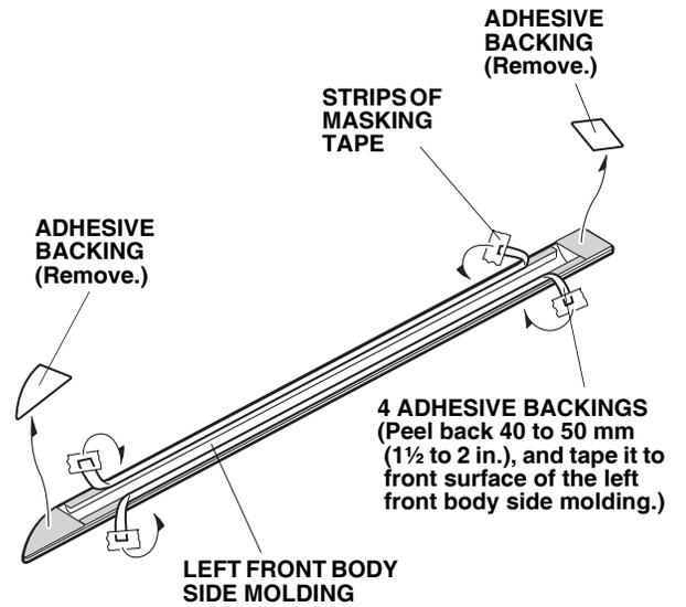
9. Align the edges of the left front body side molding with the edges of the front template, and install the left front body side molding on the left front door.
