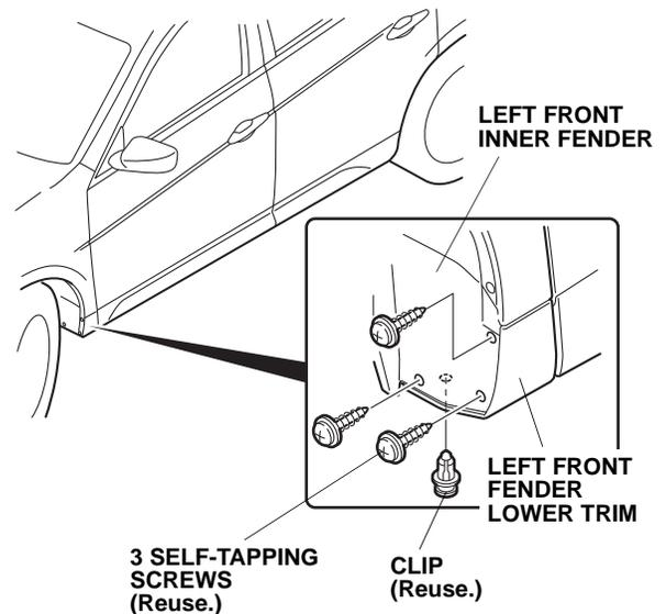
3. Pull the left front fender lower trim toward you, and remove it. The two clips will stay in the body. Set the left front lower trim aside, it will not be reused.
