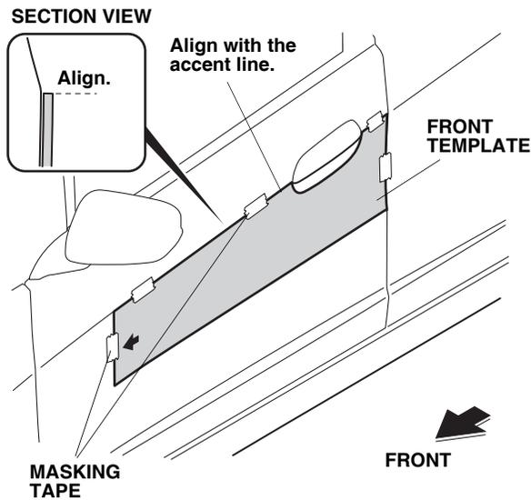
2. Peel back approximately 1½ to 2 inches of adhesive backing, and tape the ends to the front surface of the body side molding. Remove the small end pieces of adhesive backing.
