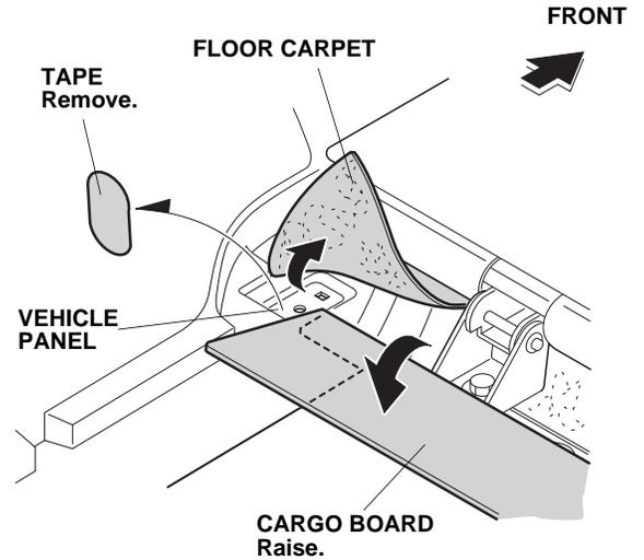
3. Remove the tape attached to the vehicle panel.
