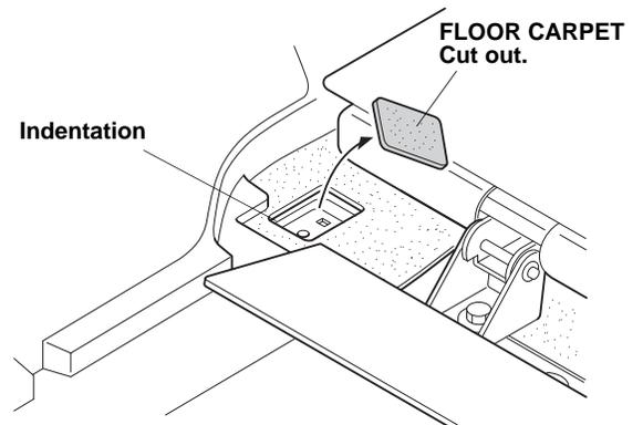
5. Fold back the carpet, and install one tie-down using the attached bolt.
