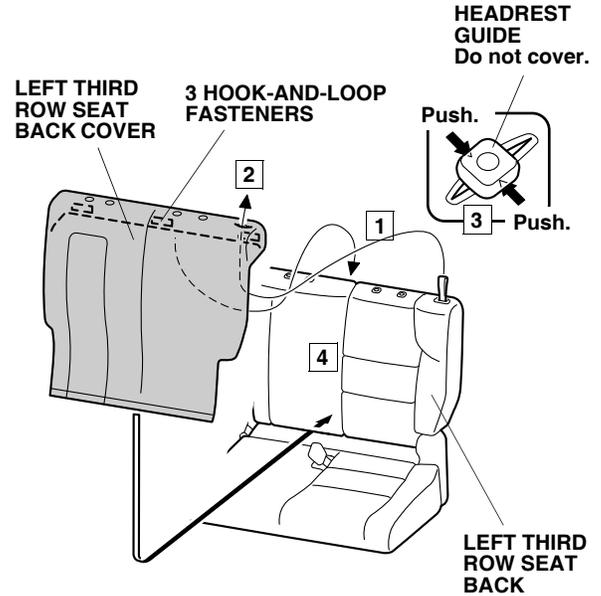
5. Fold down the left third row seat. Secure the left third row seat back cover to the left third row seat back with one hook-and-loop fastener. Return the left third row seat to its standard position.
