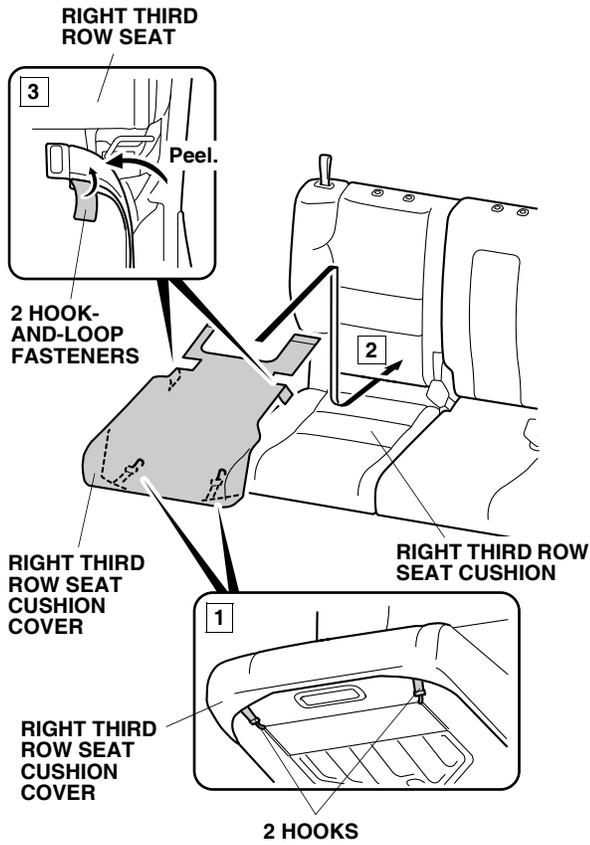
11. Secure the right third row seat cushion cover to the right third row seat cushion with the two hook-and-loop fasteners.
