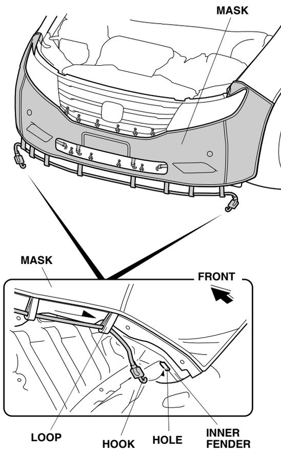
8. Secure one end of the elastic cord to the inner fender hole.
