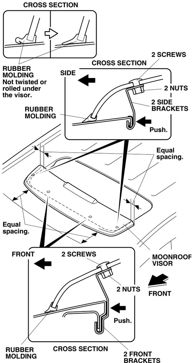
17. Tighten two screws and two nuts on each side of the vehicle first, then tighten two screws and two nuts on the front. Tighten while applying pressure so that there is no gap between the brackets and the roof panel. Torque the screws to 2 N·m (1.5 lbf-ft).
