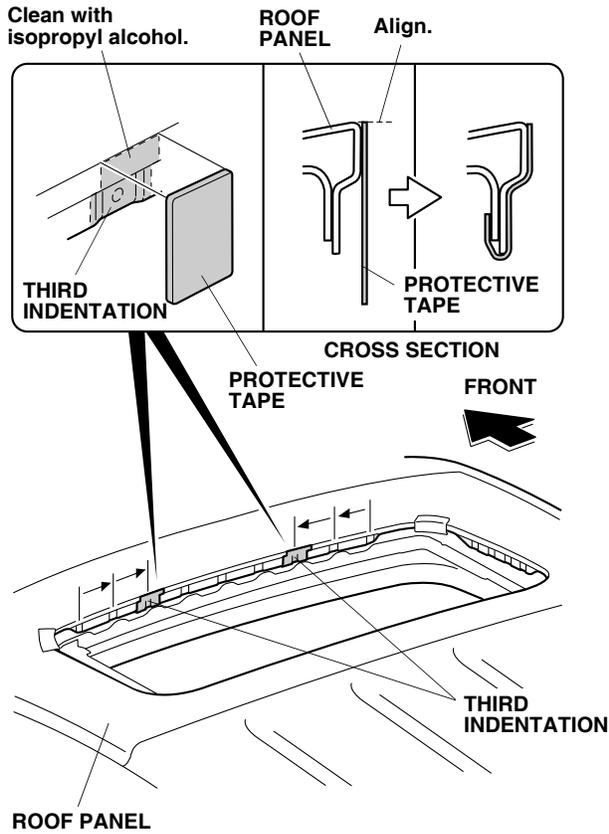
8. Remove the adhesive backing from one protective tape. Starting at the top edge, install the protective tape at the third indentation in from the right side of the moonroof opening.
