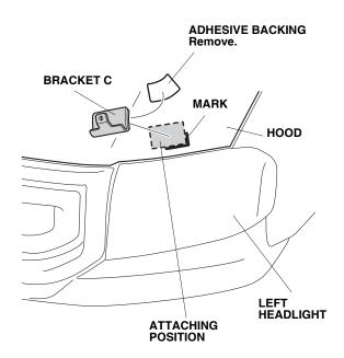
11. Reverse the template and repeat steps 7 through 10 to install bracket C on the right side of the vehicle.
