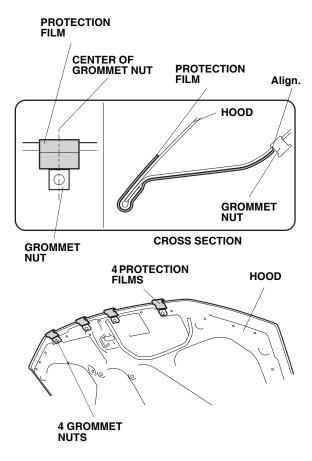
3. Remove the adhesive backings from the protection films and attach four protection films around the front of the hood as shown.
