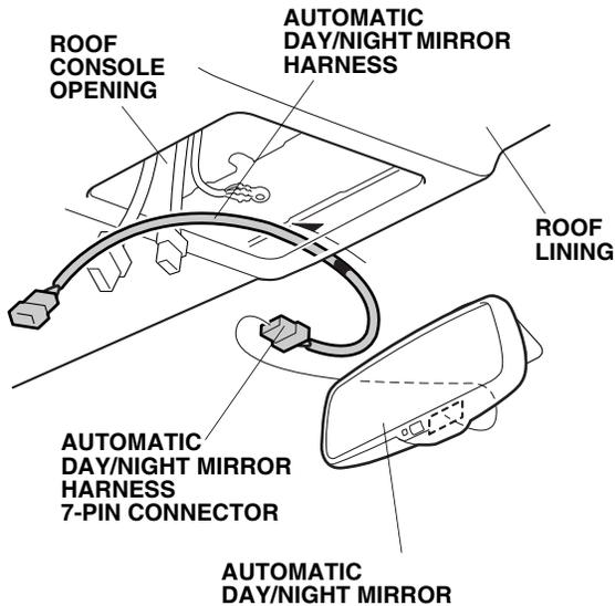
10. Align the green-taped part of the automatic day/night mirror harness with the edge of the roof lining.
