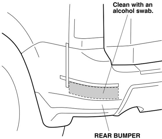
17. Remove the adhesive backing from the corner protector. Check the back of the corner protector for the correct orientation.
