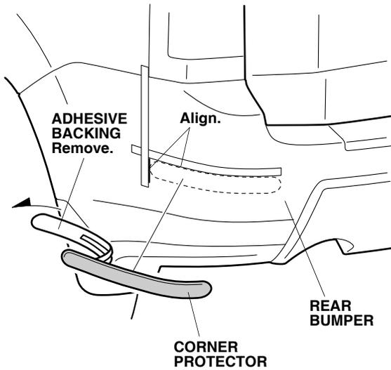
18. Align the corner protector with the masking tape and attach the corner protector to the rear bumper.
