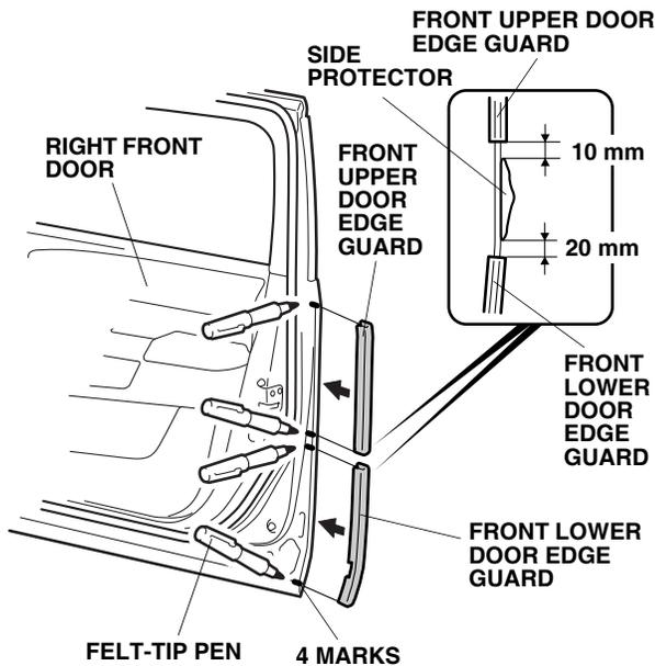
2. Measure and position the right front upper door edge guard and right front lower door edge guard on the right front door as shown.
