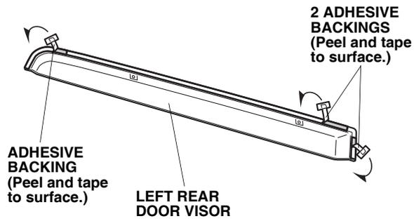
13. Using isopropyl alcohol on a shop towel, clean the door sash where the left rear door visor will attach.
