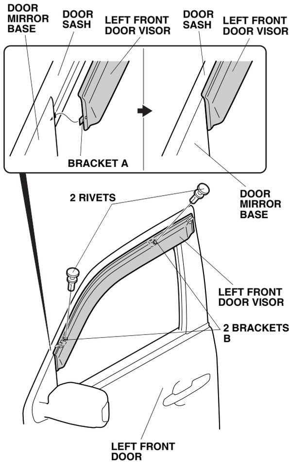
6. Align the holes on the brackets B with the holes in the left front door visor and secure it with two rivets.
