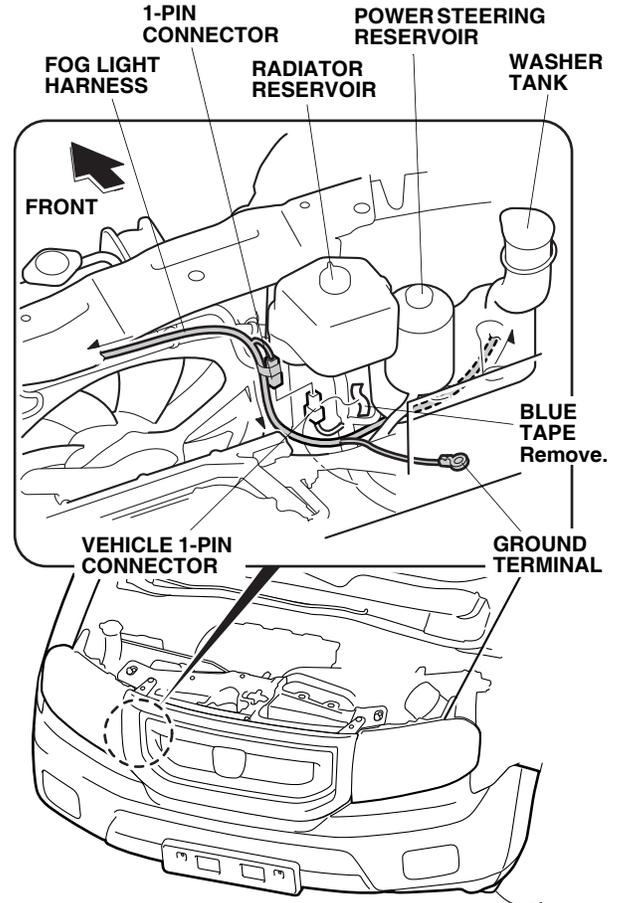
6. Plug the fog light harness 1-pin connector to the vehicle 1-pin connector.
