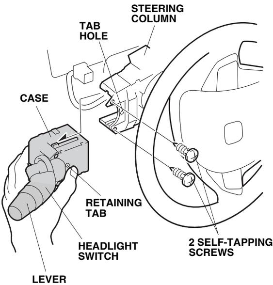
32. Install the new headlight switch on the steering column using the two self-tapping screws. Hold the case by hand, then install the new headlight switch to the steering column. Do not push on the lever when installing the case. Push on the case only and set the retaining tab to the tab hole securely.
