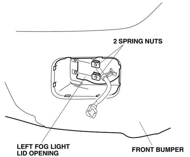
20. Plug the fog light harness 2-pin connector to the left fog light.
