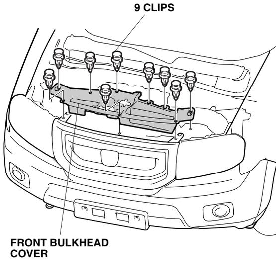
2. Remove the front bumper (nine clips, four bolts, and four self-tapping screws). Have an assistant help you when removing and installing the front bumper. If the vehicle is equipped with foglights or front corner sensors, unplug the connectors. Place the front bumper on a blanket after removal.
