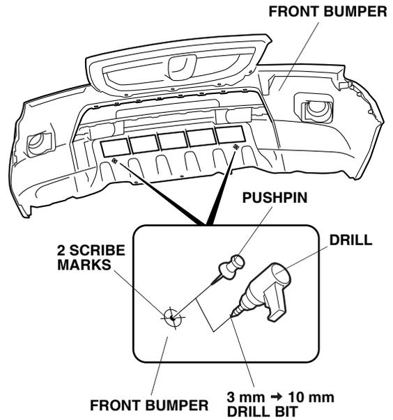
4. While wearing eye protection, first drill with a 3 mm drill bit and finish with a 10 mm drill bit. Remove all burrs.
