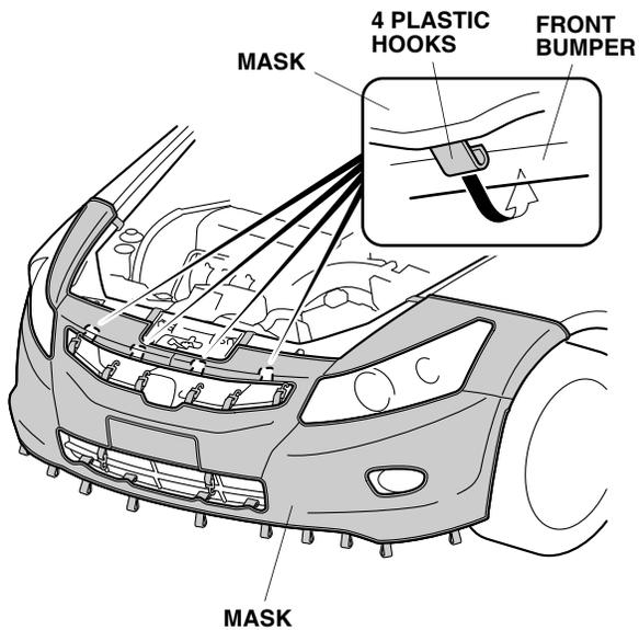
15. Attach six hooks to the inside edge of the front bumper.
