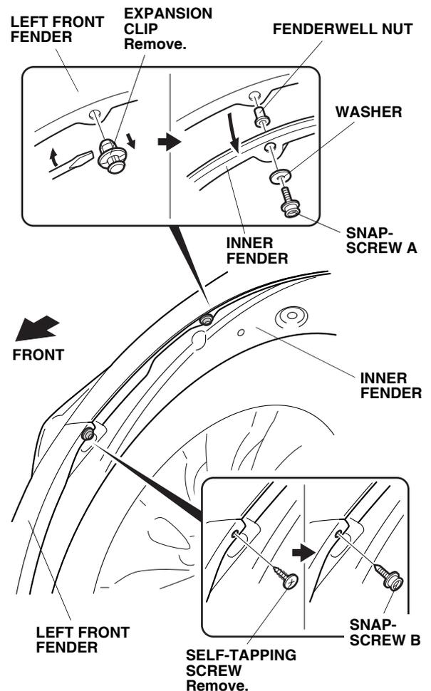
4. Pull the inner fender down, and insert one fenderwell nut into the hole in the left front fender.
